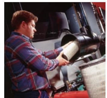
The air filter is easily accessible under the hood.
